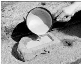
Pouring the slurry of Weld Lake pigment into the hollowed brick for drying into a powder
